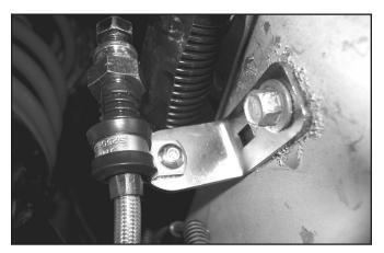
15. Using one of the supplied zip ties and rubber spacers, slide the spacer onto the tie. Loop the tie around the ABS wire at the rubber grommet, then slide the zip tie back through the spacer.
