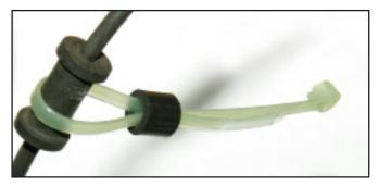
16. Secure the ABS wire to the Brake hose.
