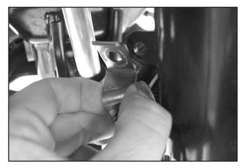
5. Disconnect the hard line. Use a flare nut wrench to avoid rounding off the fitting.
