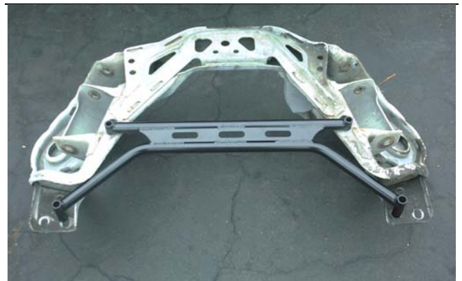
4-Point K-Brace placement on the K-member as viewed from the rear of the car
