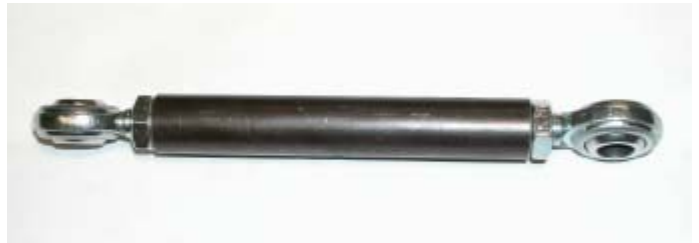
Incorrect- The rod ends are not aligned
