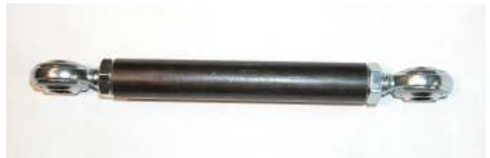
Correct- The rod ends are aligned.
