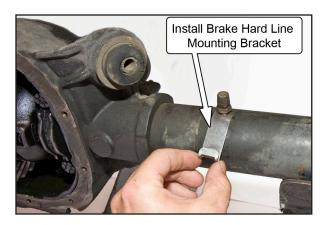
17. Slide the Passenger Side Brake Hard Line into the end of the Brake Hard Line Mounting Bracket. 18. Place one of the Brake Hard Line Retainers onto each of the Brake Hard Lines and squeeze the legs of the retainer together. Install the retainer in the orientation shown below using the supplied Sheet Metal Screws.
