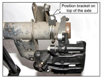
10. Wrap the hose clamp around the axle housing and loosely secure it so the position of the Brake Hose Mounting Bracket can still be adjusted.
