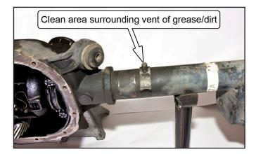
6. Remove the axle vent and the sheet metal bracket it retains on the axle using a 9/16" wrench.
