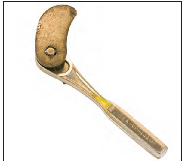
16. Fit the MM Flange Straightener on a 3/8" drive ratchet as shown.
