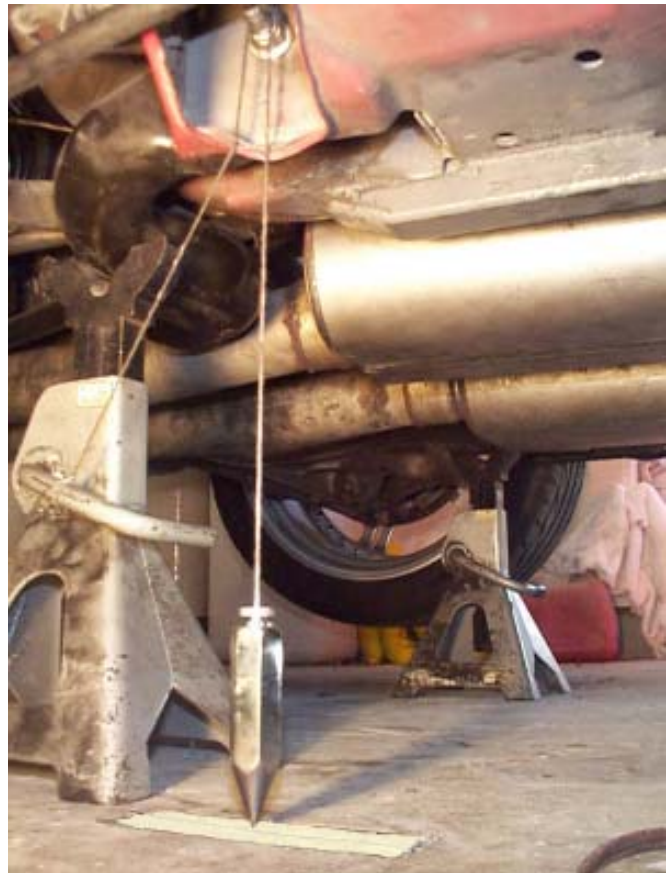
46. Wait for the plumb bob to stop swinging. Mark the position of each plumb bob by placing a small dot on the tape directly under the tip of the plumb bob.
