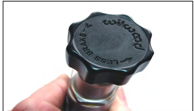
NOTE: Even at full “increase” on the knob the rear line pressure will still be slightly lower than the front line pressure. It is impossible to have higher pressure in the rear lines than the front lines with this valve.
