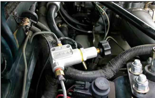
3. There is an “in” and “out” port on the Adjustable Brake Proportioning Valve. The line coming from the master cylinder connects to the “in” port and the line going to the rear brakes goes to the “out” port.
