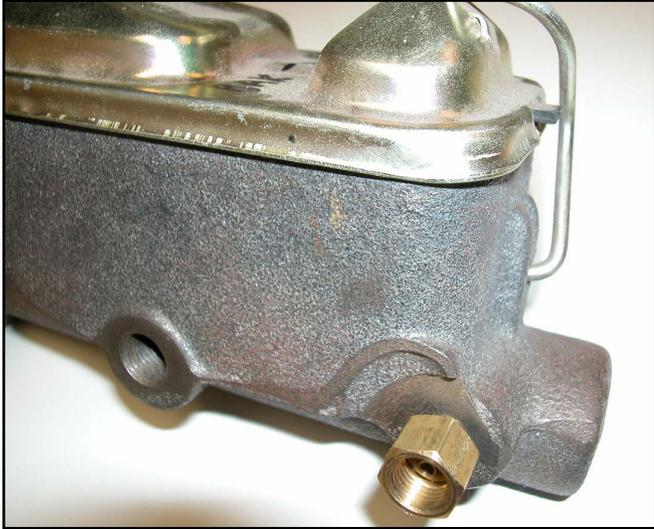
8. Thread the rearward line directly into the rear port. Tighten firmly (~14 ft-lbs). Use a flare wrench to avoid rounding off brake fittings.
