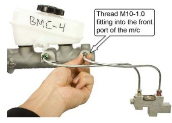
5. Thread the opposite end of the brake hard line installed in Step 4 into the front port of the stock proportioning valve (7/16-24 fitting).
