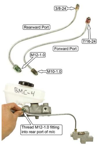
3. Thread the free end of the brake hard line installed in Step 2 into the rear port of the stock proportioning valve (3/8-24 fitting).
