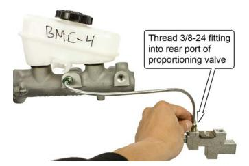
4. Thread the M10-1.0 bubble flare end of the "Forward Port" labeled brake hard line into the front port of the master cylinder. Position the free end of the hard line above the stock proportioning valve.
