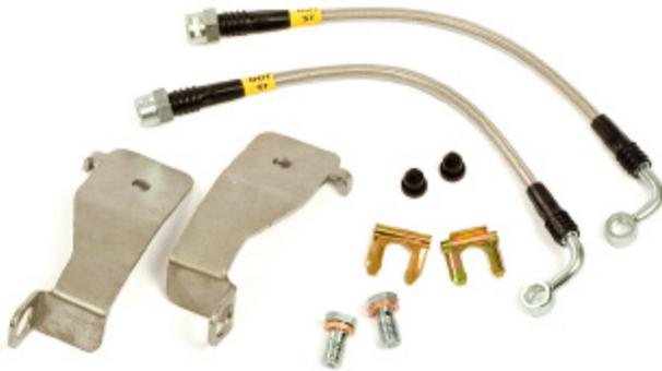
Maximum Motorsports DOT approved braided stainless steel brake hoses provide better performance because their Teflon lining does not expand under pressure like a typical rubber line will. Stainless steel hoses will provide quicker braking response, improved modulation, and a firmer brake pedal.
