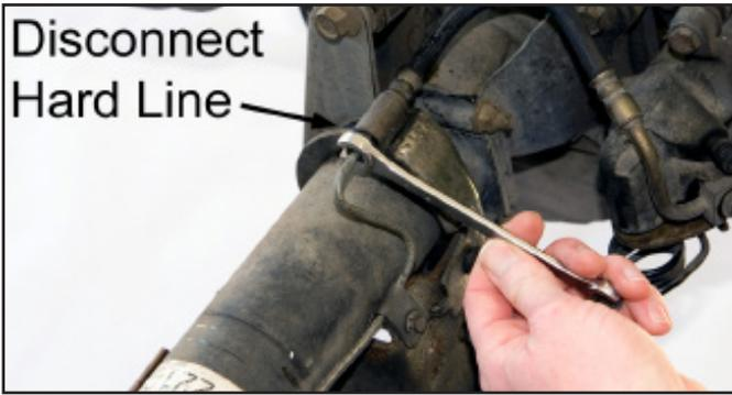
*NOTE: Use a plug to cap off the hard line to prevent brake fluid loss.*
