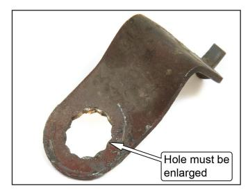
Insert the MM hose fitting through the chassis bracket until the 'E clip' seats against the bracket.
