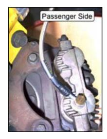
11. Torque the fluid bolt at the caliper to 12-14 ft-lb while holding the black plastic strain relief of the hose to keep the hose from rotating. 12. Turn the steering wheel back to center. On both sides of the car, gently push the hose toward the center of the car with one finger. Tighten the flare-nut on the chassis' hard line into the MM hose end. Use a flare-nut wrench to avoid rounding off the flare-nut.
