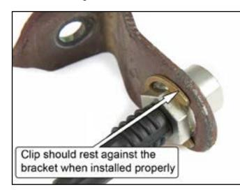
NOTE: For 1979-86 and 1987-93 4 cylinder vehicles, the hole in the bracket must be enlarged to accommodate the brake hose.
