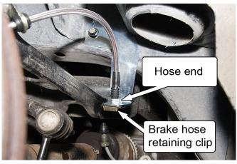
10. Route the MM Stainless Steel Brake Hose under the upper control arm and to the brake caliper. Attach the hose to the caliper using the supplied fluid bolt and crush washers. Use one crush washer on each side of the banjo fitting. Snug the fluid bolt by hand for now, as the line may still need to be slightly rotated for proper positioning.
