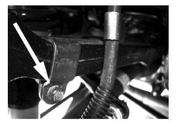
Disconnect the OEM brake hose from the brake caliper. Use a 10mm wrench or socket to remove the stock fluid bolt.
