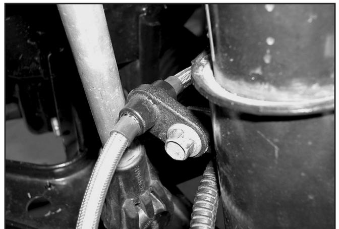
12. Install the new supplied frame rail bracket.
