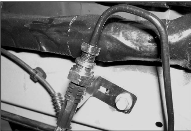
14. Secure the brake hose to the frame rail bracket using the supplied loop clamp and Allen head screw.
