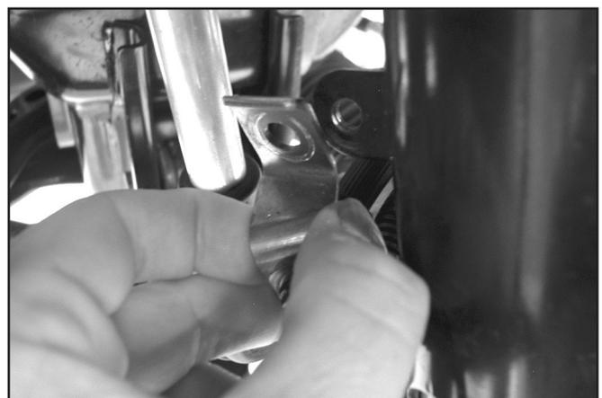
5. Disconnect the hard line. Use a flare nut wrench to avoid rounding off the fitting.
