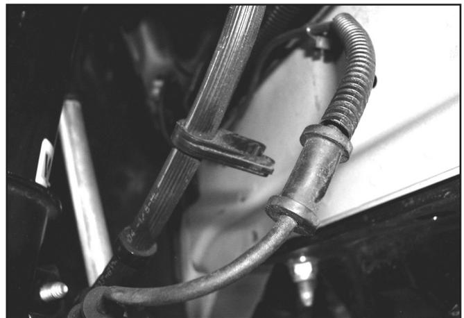
4. Unbolt the stock retainer bracket from the strut body.
