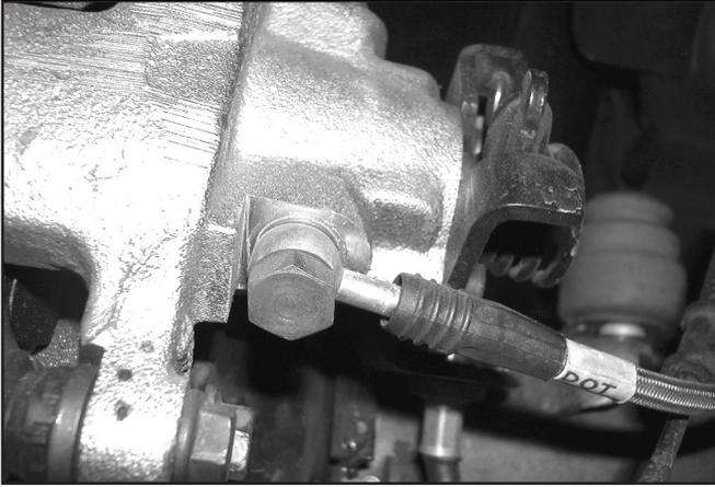
11. Torque the fluid bolt to 12-14 ft-lbs.
