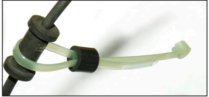
14. Secure the ABS wire to the Brake hose.
