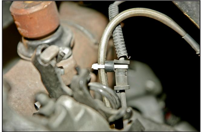
15. Snap the ABS wire into place in the frame rail mounting bracket.
