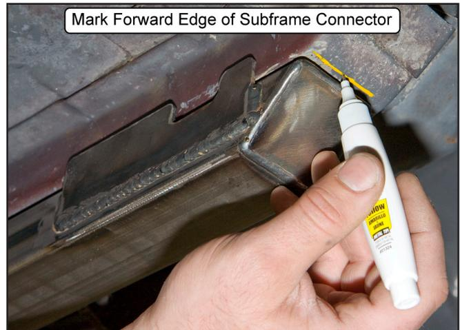
15. Push the front of the subframe connector towards the center of the car, so that the Forward Side Plate is tight against the outboard side of the car's front subframe.
