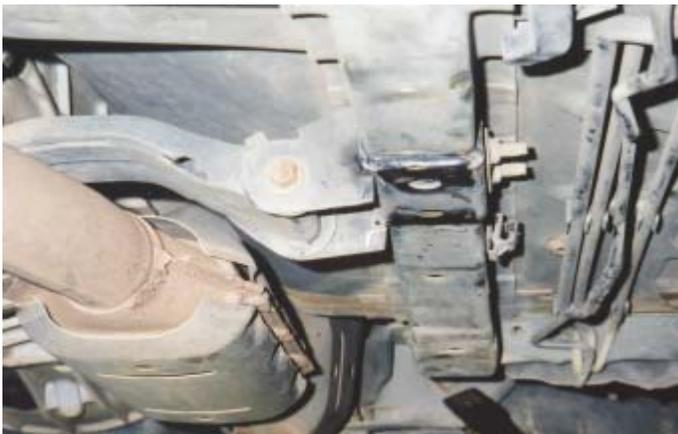
3. After welding the subframe connectors in place, weld the transmission mounts to the subframe connectors. Full length (MMFL-3) subframe connector is shown in the picture below. Standard length subframe connectors attach similarly.
