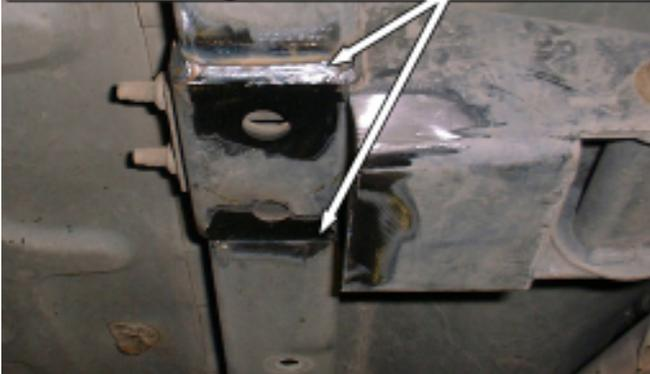
2. Notch the passenger side transmission mount so that the subframe connector will sit flush and square to the front subframe.
