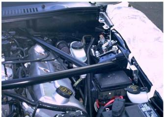
5. Check for clearance around the air inlet tube.
