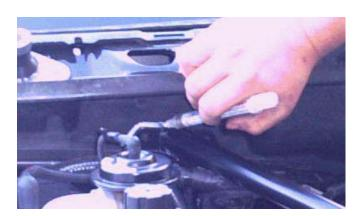
7. Remove the Strut Tower Brace.
