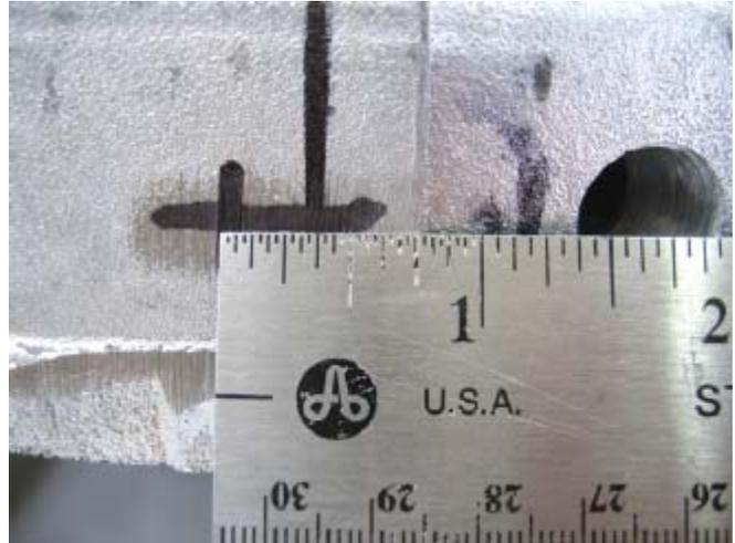
85. Use a center punch to mark the center of the "X".
