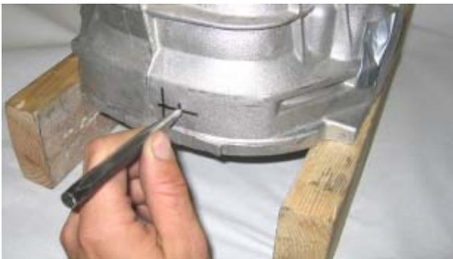
66. Using a  $\frac{1}{8}$ " drill bit, drill a pilot hole through the center punched mark.
