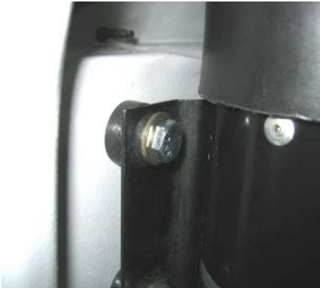
114. Place the differential oil pump in its final mounting location so that the four bolts pass through the holes drilled in Step 111.
