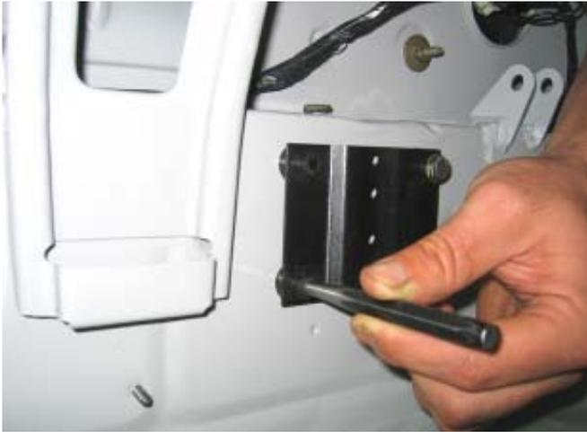
111. Starting with a small pilot hole, drill the center punched marks out to a 1/4" diameter hole.
