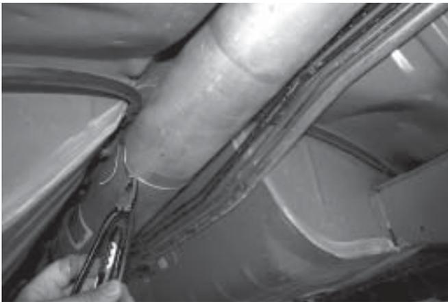
24. Unbolt the ABS sensors from each side of the differential housing. These attachment bolts have a head with both an external hex and an internal Torx.
