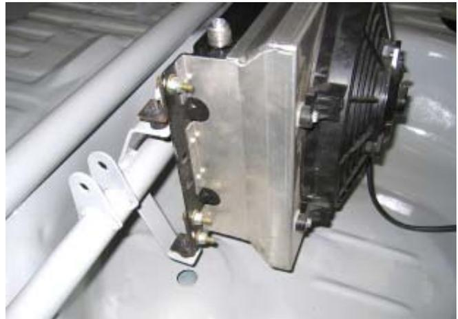
102. Attach four of the provided rubber isolators to the four oil cooler mounting tabs made in the previous step, with one 3/16" fender washer and one M4 nylock nut on each rubber isolator.
