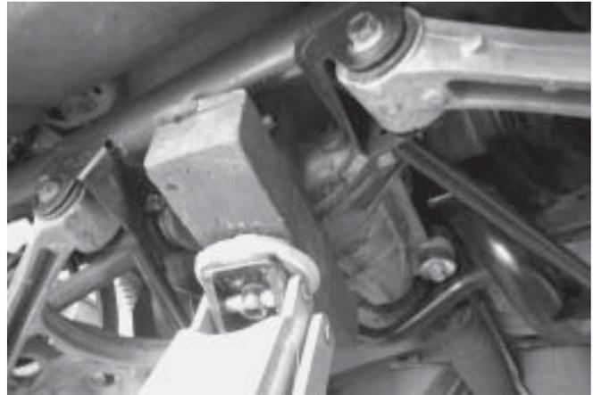
26. Remove the two mounting bolts, located on the differential cover, that attach the cover to the rearward differential bushing.
