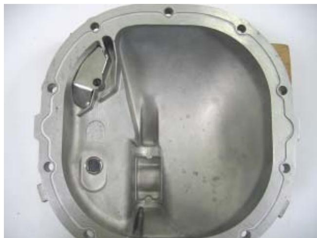
40. Locate the raised casting circle directly above the differential fill plug. Center punch a mark 3/16" above the center of the casting circle.
