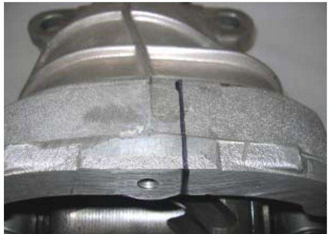
61. Stand the differential case up on two blocks of wood with the bottom of the case facing towards you.
