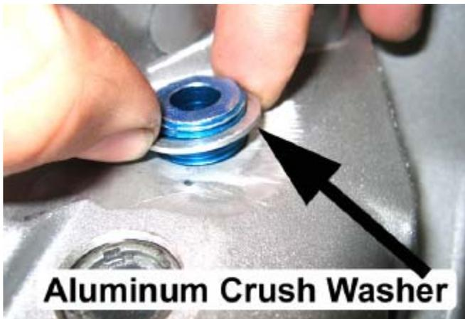
51. Place a few drops of the supplied Blue Loctite® on the threads of bulkhead fitting, adjacent to the aluminum crush washer installed in the previous step.
