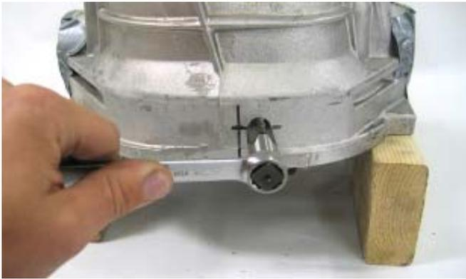
71. Periodically unthread the tap and clean the threads of any metal chips. After cleaning, apply more lubricant to the tap.
