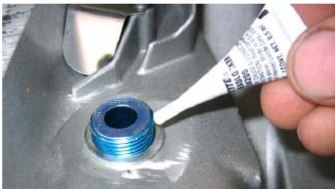
52. Thread the supplied AN blue aluminum nut onto the bulkhead fitting.
