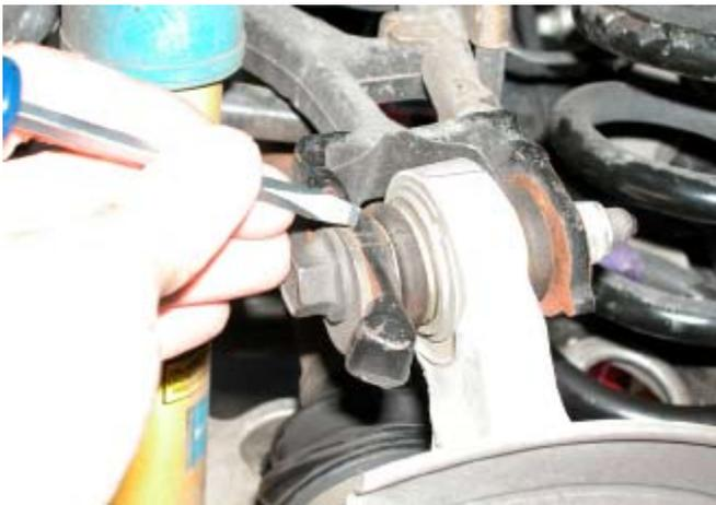
12. Loosen the upper and lower spindle mounting bolts.
