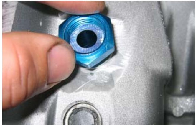
53. Tighten the nut as much as possible by hand, and then use a wrench to tighten the nut a further 3/8 of a turn.
