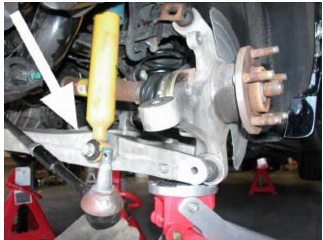
16. Pull out the upper spindle-to-control arm mounting bolt and carefully remove the axle half-shaft/spindle assembly. Take care to avoid damage to the differential seal.
