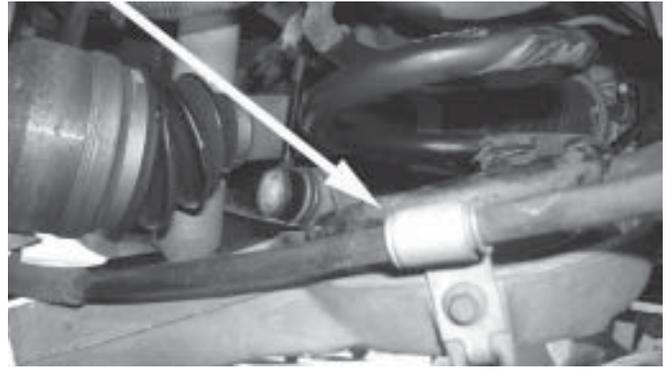
5. Remove the parking brake cable housing retaining clip on each caliper.
