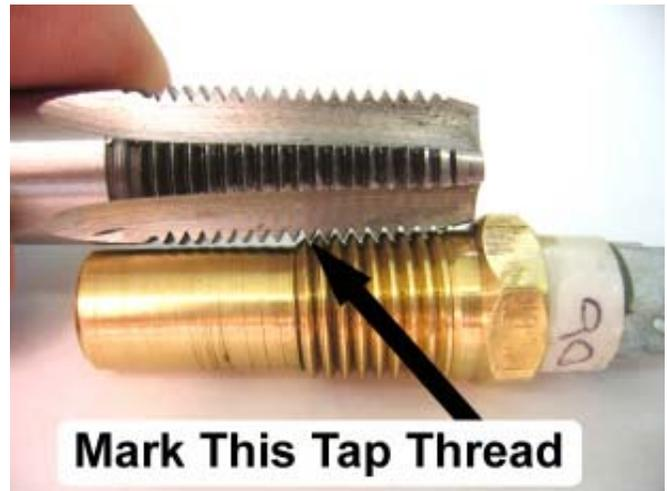
77. Count three full threads on the 1/4" NPT pipe tap, above the mark previously made, and wrap a piece of masking tape around the tap. The masking tape should be wrapped above the third thread. The 1/4" NPT tap is now ready for use.
