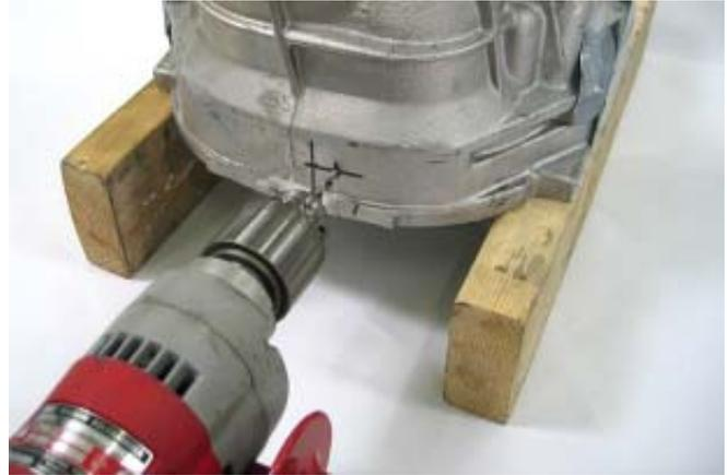
67. Carefully enlarge the hole, using larger and larger drill bits, until the final size is drilled with a  $\frac{9}{16}$ " drill bit.
