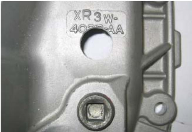
43. Deburr both faces of the hole, using a hand file or deburring tool.
