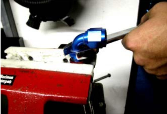
165. Make sure your mark at the end of the socket has not moved more than 1/16", if it has return to Step 161 and repeat the process.
