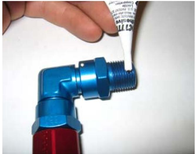
168. Thread the fitting into the bottom of the differential case and hand tighten.
