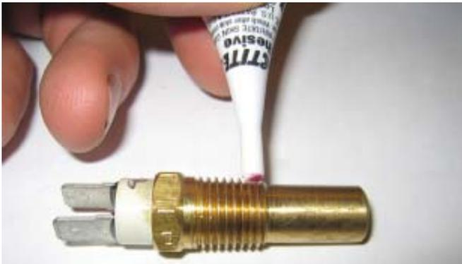
174. Thread the switch into the previously tapped hole in the bottom of the differential case, and hand tighten.
