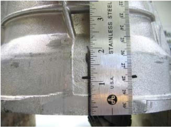
64. Next, measure over  $\frac{1}{2}$ " to the right of the vertical line, along the horizontal line made in the previous step, and make a small, vertical mark.
