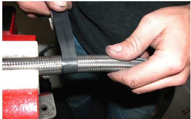
6. Squarely cut through the tape-wrapped sections of the hose using a sharp 32 TPI (or finer) hacksaw blade.
