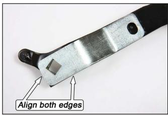
Once the edges are aligned, tape the MM Clutch Pedal Adjuster to the OEM clutch pedal lever as shown. This will ensure that the alignment of the part doesn't change while locating the transfer punch in the next step.
