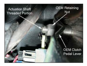
Remove the retaining clip from the clutch lock-out switch shaft. Remove the OEM clutch pedal lever from the square-shaped shoulder on the actuation shaft. Rotate the OEM clutch pedal lever to facilitate the removal of the clutch pedal lock-out switch arm. Remove OEM clutch pedal lever from the car.
