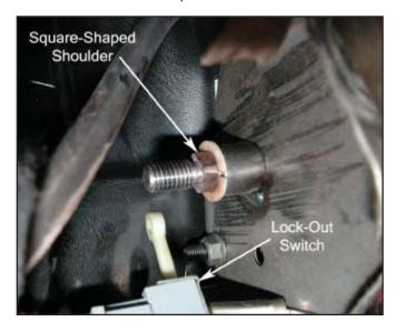
4. Place the arm as shown and line up the lower edges of the MM Clutch Pedal Adjuster with the edges of the OEM clutch pedal lever. The alignment of the edges does not have to be perfect.
