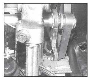
The Maximum Motorsports clutch quadrant is designed to clear the quadrant limit bracket and maintain the OEM at-rest position of the actuation shaft. If using a Maximum Motorsports clutch quadrant, no modifications of the quadrant limit bracket are necessary (See picture below).
