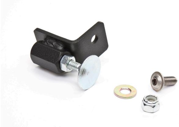
Tilton multi-disc racing clutches require a properly adjusted pedal stop to prevent damage to the clutch assembly. This adjustable pedal stop limits travel of the clutch pedal to prevent over-stroking the pressure plate. It must be adjusted to allow just enough pedal travel to disengage the clutch, but no more. MM designed this product specifically to fit the stock clutch pedal of 2005-2014 Mustangs.
