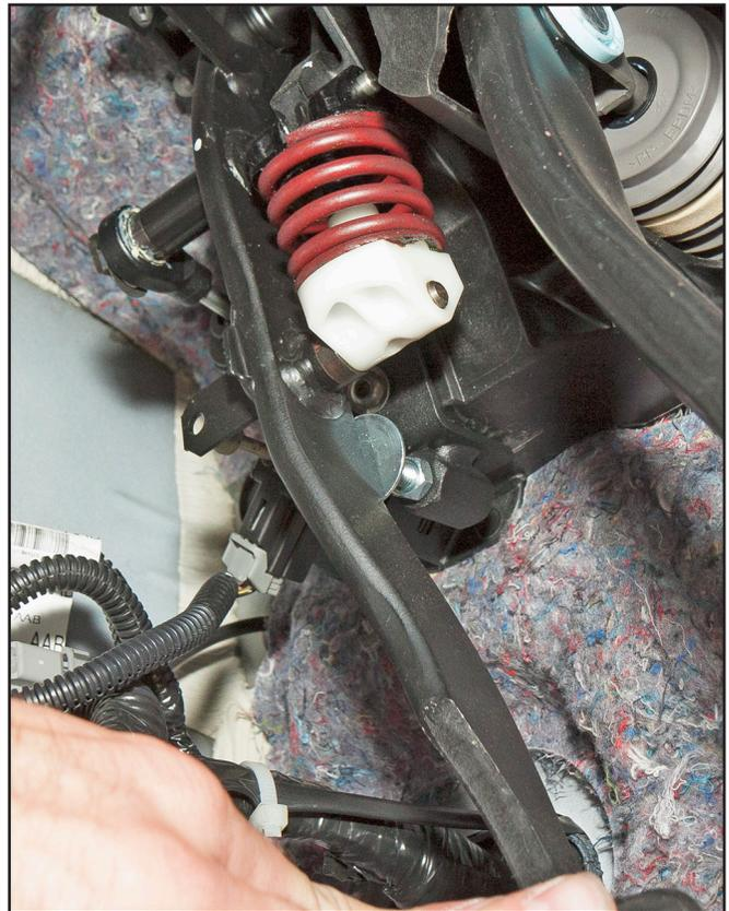
25. After adjusting the MM Clutch Pedal Stop, reset the clutch pedal position switch. The grey plunger is extendable; pull it out until you hear its ratcheting mechanism release.
