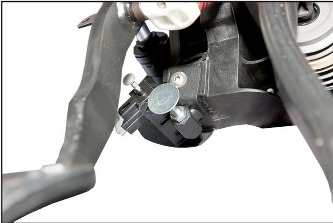
11. Install the button-head socket cap screw through the MM Clutch Stop, and then through the pedal bracket assembly. Install the washer and nut. Torque the button-head socket cap screw (5/32" Allen) and nut (7/16" socket) to 16 Nm (12 lb-ft). *Do not over-tighten!*
