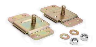
Thank you for purchasing this Maximum Motorsports' Coyote Swap Firewall-Clearance Motor Mount Adapters. These MM Motor Mount Adapters relocate the engine about 0.7" forward from the location set by standard 4.6L motor mounts. This provides room for the CMCV vacuum motors of Gen 2 (2015-2017) and Gen 3 (2018+) Coyote engines to clear the 1979-2004 Mustang firewall.
