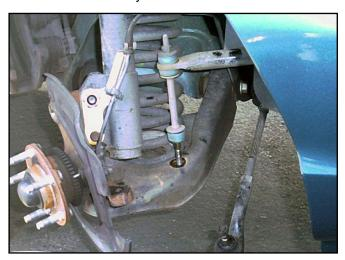
7. If the car is equipped with ABS, carefully unhook the sensor's wire from the mounting bracket on the strut to get enough slack in the wire to remove the sensor from the spindle. Remove the sensor-to-spindle bolt, and carefully remove the sensor from the spindle. Remove the mounting bracket from the strut.
