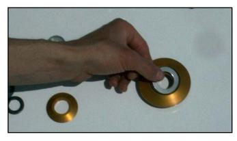
33. Set the Thrust Cone onto the top of the Upper Spring Perch.
