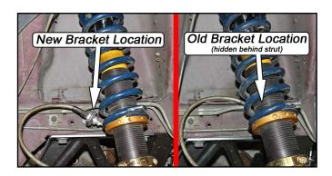
Follow the instructions below to relocate the bracket. Passenger side shown.
