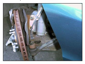
6. Disconnect the swaybar end-link from the control arm.
