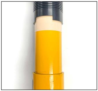
28. For Tokico Struts with a swaged cap, re-install the cap at this time. Using a piece of wood and a hammer, drive the cap back into place. Be sure to move the wood block around in order to drive the cap into place evenly.
