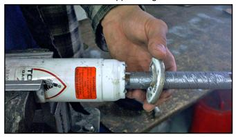
21 . Add another wrap of duct tape on the 1/8" of strut shaft that was hidden by the Tokico upper flange. Use a file to remove the exposed spot welds on the top of the strut housing. It is critical to make the spot welds smooth to avoid damage to the bumpstops. Skip to Step 26.
