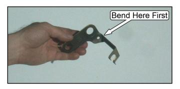
48. Then carefully bend it upward near the end where the wire attaches.
