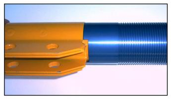
NOTE: Due to manufacturing irregularities the diameter of strut housings varies from batch to batch. Our coil-over threaded sleeves accommodate inconsistencies in the diameter of the strut housing by installing a PTFE Shim to fill in any gap between the strut housing and our threaded coil-over sleeve. Reducing any gap to a minimum reduces the possibility of noise when driving.
