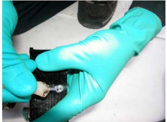
11. Place the greased urethane bushings onto the swaybar, and slide the new Universal U-brackets onto the urethane bushings.
