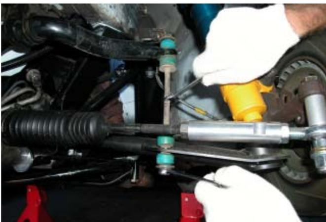
4. Remove the four bolts which hold the swaybar pivot U-brackets to the chassis. Hold the swaybar while removing the bolts to prevent it from falling.
