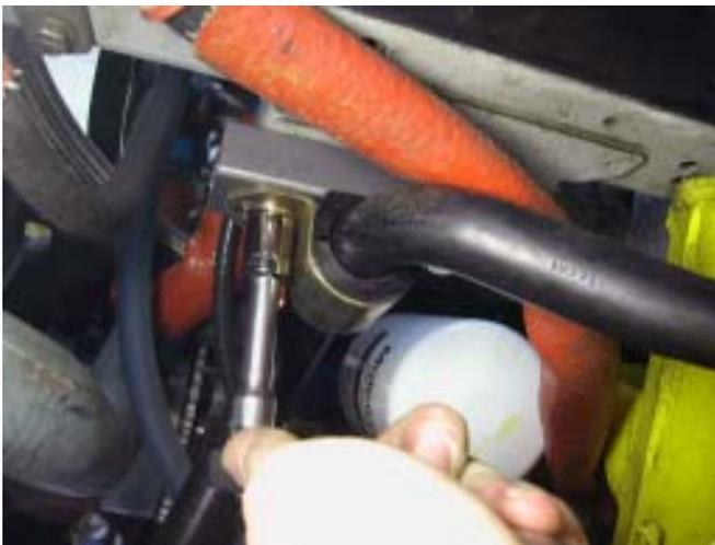
16. Reattach the endlinks to the swaybar. Be careful not to overtighten and excessively crush the endlink bushings.
