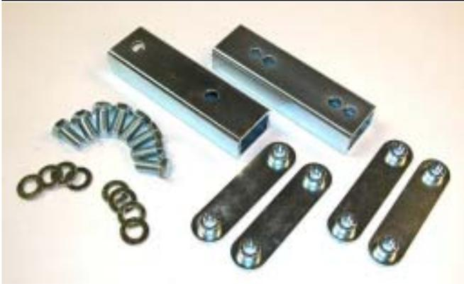
The MM Front Swaybar Relocation Kit allows the option of moving the front swaybar forward 0.6" or 1.1". This keeps the swaybar endlinks in alignment with the control arms when the front wheels have been moved forward with an MM K-member and MM Forward Offset Control Arms. The MM Front Swaybar Relocation Kit can also be used with other aftermarket K-members that move the wheels forward. The use of this kit requires a set of universal swaybar U-brackets (P/N 6-1124 to 6-1137)
