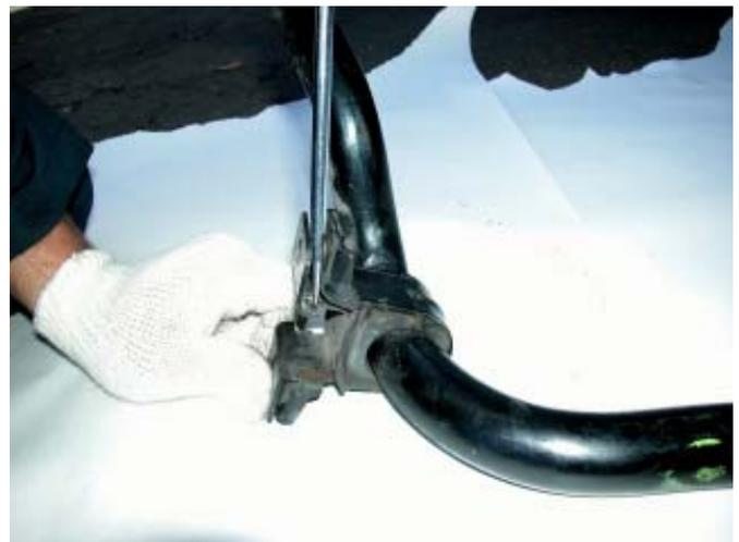
6. Remove rubber swaybar pivot bushings from the swaybar.
