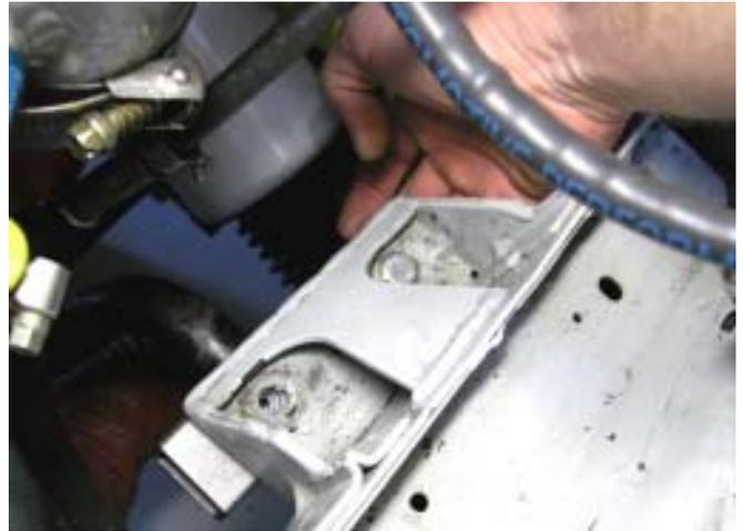
10. Liberally grease the inside of the universal front sway bar bushings with the supplied Prothane Super Grease. Coat 100% of the bushing surface in contact with the swaybar.
