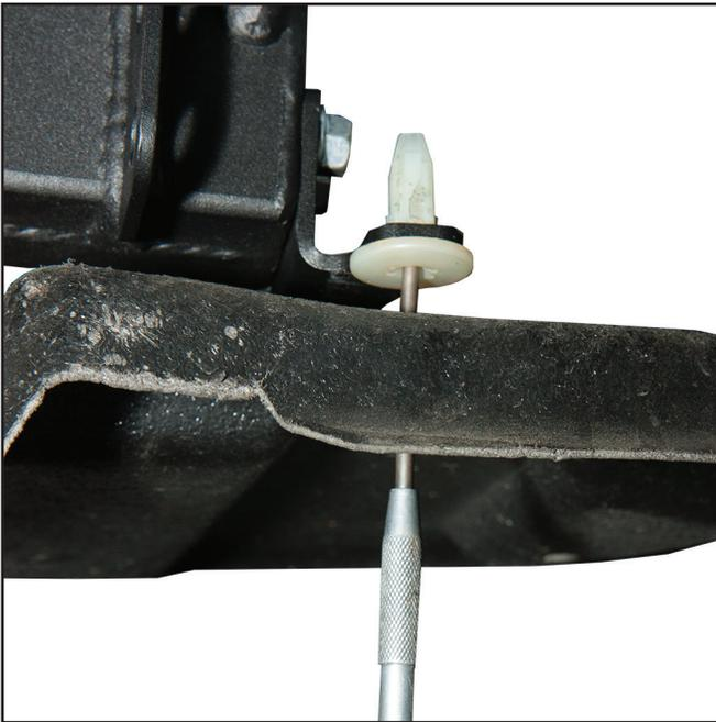
29. (2011-14 ONLY) Attach the air deflector to the L-brackets using two of the remaining fasteners. There will be one remaining fastener that is no longer used and can be discarded.
