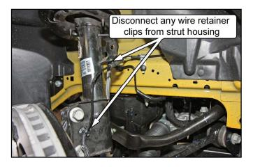
5. Disconnect the front stabilizer bar link from the strut housing. Use a 17mm wrench on the flats of the stud to stop it from rotating and an 18mm socket to remove the nut.
