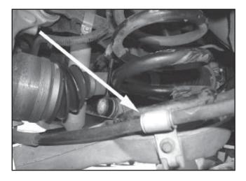
Make sure the parking brake is not set, and then remove the parking brake cable housing retaining clip on each caliper.
