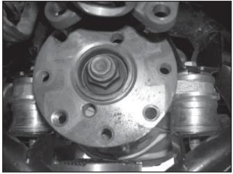
NOTE: At least one Steel Shim Spacer must be present between each differential crossmember mounting tab and the installed aluminum Front Differential Mount Spacers.
