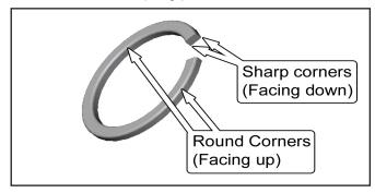
28. Orient the circlip with the sharp corners facing down toward the spring perch. Slide the circlip over the top of the shock shaft, past the threaded section, until it reaches the groove above the larger diameter portion of the shaft. The circlip should be tight around the shock shaft. If the circlip is loose on the shock shaft, then it has been damaged. Call Maximum Motorsports for a replacement circlip.
