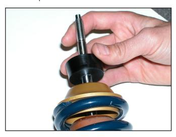
30. Completely coat the inside of the pivot socket with the supplied grease.
