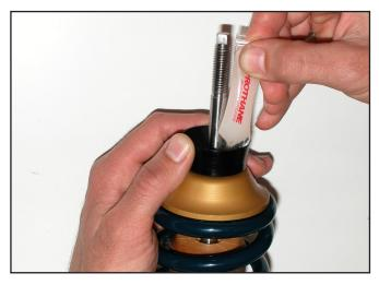
31. Place one of the Delrin pivot balls on the shock shaft with the curved side facing down toward the aluminum pivot socket.
