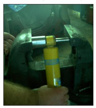
13. Use a similar process to remove the rubber bushings from each shock eyelet. Select a socket that is large enough to accept the rubber bushing into its center, but will still support the steel eye of the lower shock mount. Then select a smaller deep socket that will be able to push the rubber bushing out of the steel eye.
