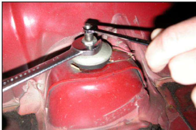
30. Raise the lower spring perch until the spring just contacts the upper and lower spring perches.
