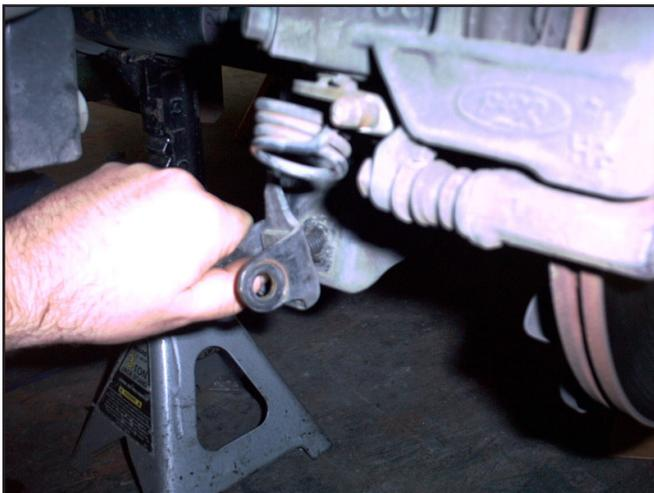
15. Install the MM lower shock mount onto the passenger side of the axle. Insert the 1/2" bolt (no washer) through the lower hole, with the bolt head facing the rear of the car. Next, place the
