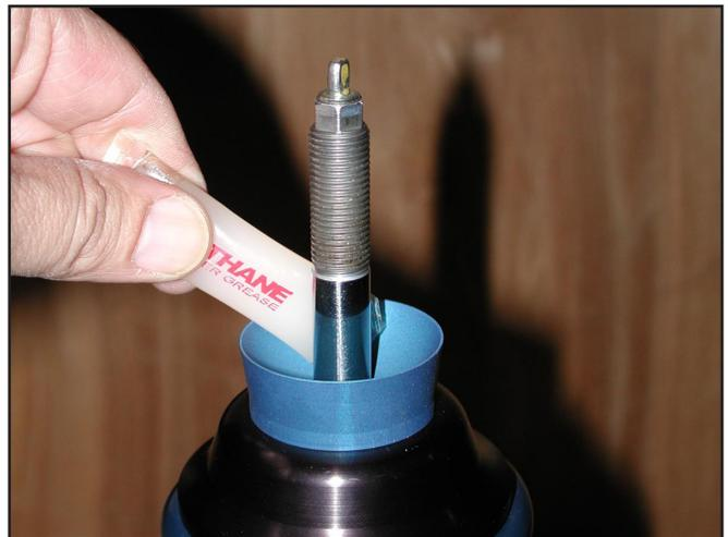
25. Place one of the Delrin pivot balls on the shock piston rod with the curved side facing down toward the aluminum pivot socket.
