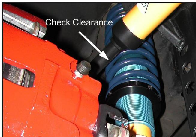
32. Repeat Steps 26 - 31 to install the completed coil-over assembly into the driver's side of the car.
