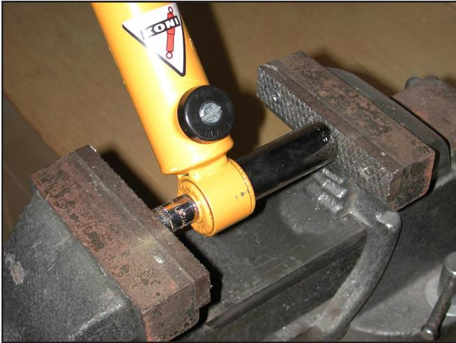
13. Use a similar process to remove the rubber bushings from each shock eyelet. Select a socket that is large enough to accept the rubber bushing into its center, but will still support the steel eye of the lower shock mount. Then select a smaller deep socket that will be able to push the rubber bushing out of the steel eye.
