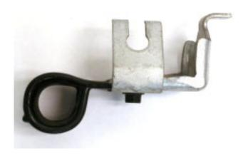
13. Flip the Parking Brake Bracket 180 degrees and place the ABS bracket on top of the parking brake bracket.
