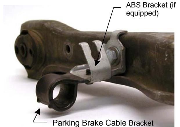
6. If so equipped, unclip the ABS wire from the bracket.
