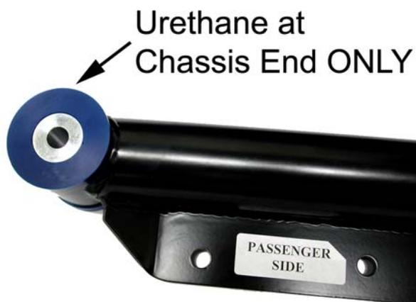
17. Apply a liberal coating of grease to the outside flange of the installed urethane bushings, where they will contact the chassis.
