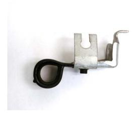
13. Flip the Parking Brake Cable Bracket 180 degrees and place the ABS Bracket on top of the Parking Brake Cable Bracket.
