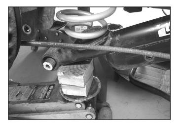
9. Remove the control arm pivot bolt from the chassis and remove the control arm from the car.
