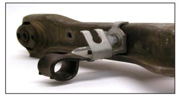
24. If so equipped, unclip the ABS sensor wire from the parking brake cable bracket.
