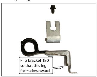
36. Attach the ABS bracket with the original screw, coming down from above.
