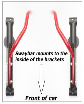
49. If needed, use the supplied Swaybar Spacer Plate. There is a surprisingly wide production tolerance range for Mustang rear swaybars, both OEM Ford and aftermarket. The MM Swaybar Spacer Plate helps mount swaybars that were made on the narrow end of the production tolerance. It does not matter which control arm the spacer plate is mounted with.
