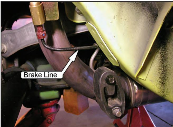
26. Remove the rubber Exhaust Hanger.
