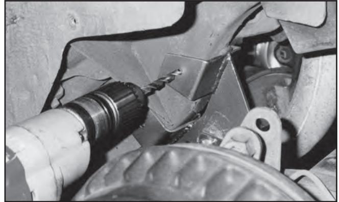
35. Slide (1) 5/16" X 3 1/4" G8 bolt through the hole you just drilled and put a 5/16" Nylock nut on, finger tight.
