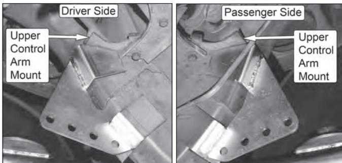
*NOTE: Check for interference between the passenger side Chassis Mount and the fuel line. Along the inside of the frame rail there is a small clip holding the fuel line to the frame rail which may need to be removed.*
