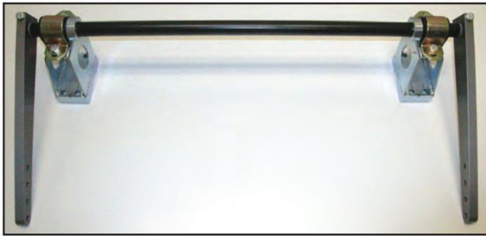
20. Bolt the Installation Plates on the outside of each Swaybar Arm. Use (4) 3/8" X 1" G5 bolts and (4) 3/8" AN Washer, placing one under the head of each bolt. Lightly tighten the bolts. The Installation Plate will be used to keep the Chassis Brackets in the correct position and square on the car during installation. The Installation Plate is installed such that the remaining open hole is positioned away from the Swaybar Tube, towards the end of the arms.
