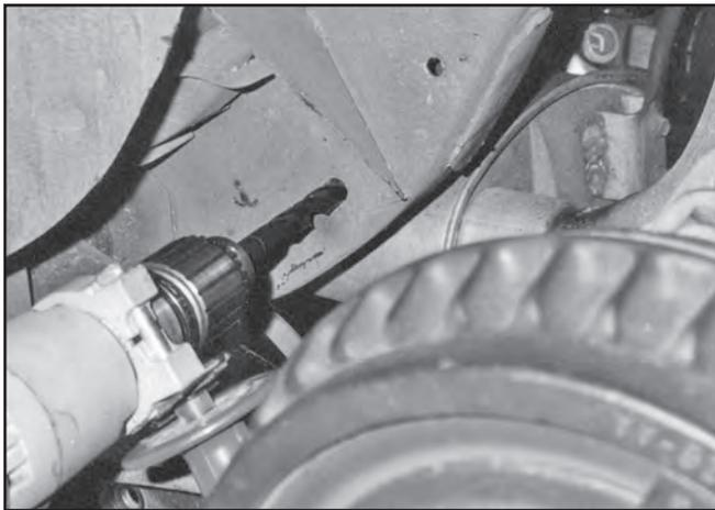
40. The frame insert tubes must be cut to the proper length for your car. Determine the proper length for **each** tube by inserting a bolt, screwdriver or caliper into the hole you drilled until it touches the inside of the inboard side of the frame rail. Carefully record the depth at the **outside** edge of the frame rail.
