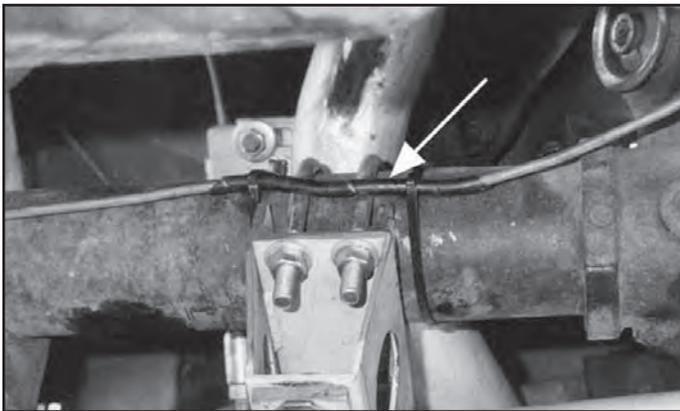
51. Remove the Installation Plates.
