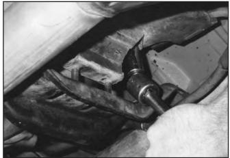
32. Bolt the transmission crossmember to the transmission mount. Slide the bolts between the transmission crossmember and the chassis in place. Lower the floor-jack supporting the transmission.
