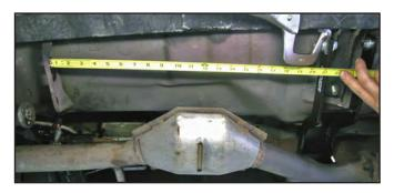
21. Using an angle finder, measure the angle of the torque arm rearwards of the forward most bend.
