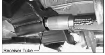
15. The rearward edge of the urethane (closest to the TA) must be flush with the rearward edge of the Receiver Tube to provide proper clearance during suspension movement, and for the grease fitting to lubricate the Urethane Bushings properly.
