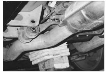
8. Lower and rotate the transmission crossmember to provide access to the two bolts holding the transmission mount to the transmission. Remove these bolts to allow the H-pipe to drop down away from the chassis during installation.
