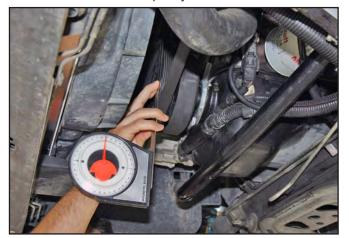
40. The goal is to make the pinion angle of the differential match the transmission output shaft angle. Each 2" shim will add or subtract 1/2 degree. Do not be surprised if you have to raise the front of the differ-
