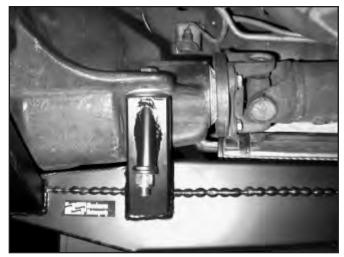
38. Measure the pinion angle. The easiest way to do this is to place an angle finder on a straight edge and place the straight edge on the driveshaft mounting flange.
