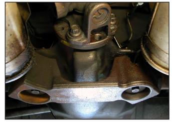
Remove the pinion snubber assembly from the bottom of the chassis (directly above the front of the differential). It is held in place with three small screws.
