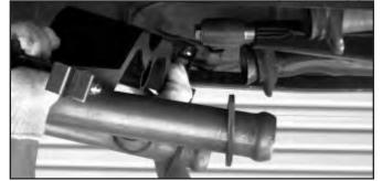
14. The TA Crossmember may now be slid rearwards while inserting the Urethane Pivot Bolt Assembly into the TA Crossmember Receiver Tube.
