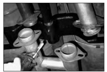
30. Cut a 3" and a 5" length of tubing the same diameter as your H-pipe tubing. Weld the 3" length of tubing onto the driver's side to extend the flange rearward. Weld the 5" length of tubing onto the passenger's side to extend that flange rearward. Shorten each tube between the flange and the muffler by the same amount the flange was moved rearward.
