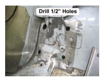
26. Reposition the driver side Weld-on Reinforcement Plate so that four pre-welded nuts on the backside of the Plate are centered over the 1/2" drilled holes. The top half of the pad should be resting flush with the floor pan and touching the inner fender well.
