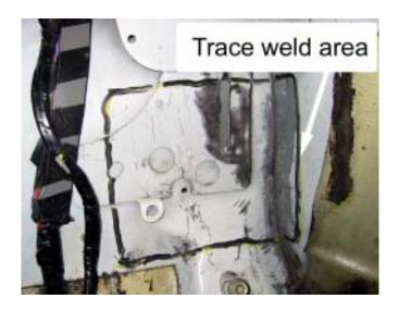
22. Using a power sander, carefully sand away any paint within ½" on either side of the outline made in the previous step. The paint must be fully removed to allow proper welding of the Weld-on Reinforcement Plate to the vehicle.
