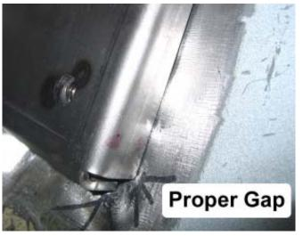
NOTE: On some vehicles the upper, outboard corner of the Weld-on Reinforcement Plates will be spaced away from the floor pan. If this occurs, place a screwdriver through the adjacent ½" hole that was drilled in Step 25 and carefully pry the sheet metal upwards to minimize the gap.
