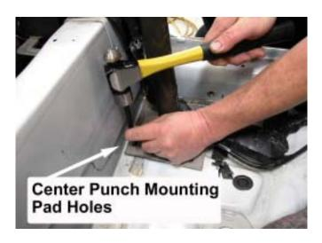
57. Put the convertible top down and slide the Main Hoop forward so that you can gain access to the center punch marks.
