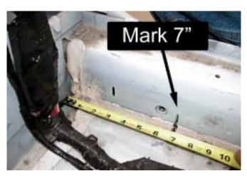
16. Again, starting at the rear corner of the driver side floor pan, make a mark 7" inward from the corner, along the rear bulkhead. Repeat for the passenger side.
