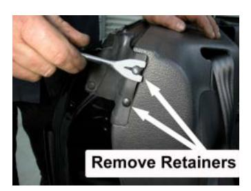
12. Begin removal of the driver and passenger rear plastic side panels by first removing the four plastic retainers holding each side panel to the vehicle. Then pull the panels away from the B-Pillar.
