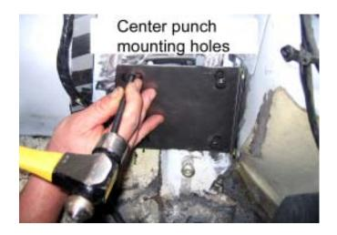
24. Using a 1/8" or similar sized drill bit, create a pilot hole at each of the center punch marks.
