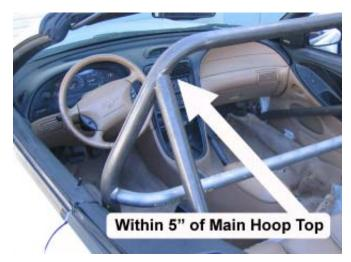
77. Use an angle finder to measure the angle of the Rear Support. If the angle is less than 30° from vertical, the Rear Support must be shortened so that the angled end can be positioned higher up on the Rear Support Pad while keeping the notched end at the same location on the Main Hoop. Be sure the car is at normal ride height and on level ground when measuring this angle.
