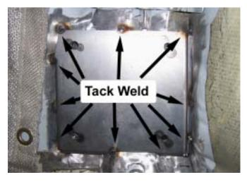
35. Starting at the top, exterior edge of the Weld-on Reinforcement Plate, begin welding the Plate to the vehicle. Continue welding the edge until you reach the gap pictured below.
