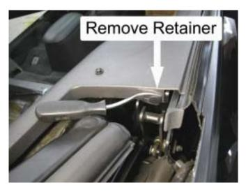
NOTE: There are two hidden clips attached to each plastic side panel, one located at the top and one located at the center of the panel where it attaches to the B-Pillar. Some effort may be required to pull the plastic side panels free from the B-Pillar.
