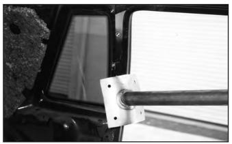
14. Slide the main hoop rearward so all mounting pads are in the correct position. The main hoop mounting pads should be centered side to side and flush with the rear seat bulkhead. Hatchback: The main hoop with the driver-side rear brace will set in the car as a tripod.
