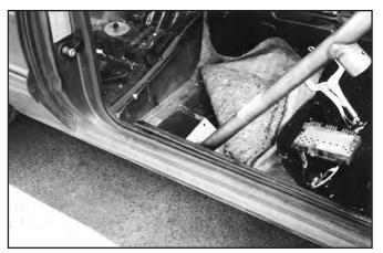
12. Pull the main hoop forward so the mounting pads 13. Keeping the main hoop mounting pads in about the same forward position, tilt the main hoop rearward so the rear brace mounting pads move toward the rear wheel well housings.
