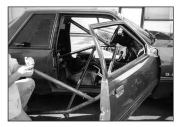
9. Maneuver the driver side of the main hoop up and over the center console, keeping the rearmounting pad behind the center console.
