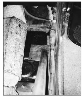
18. Close the doors and check for arm-rest clearance. The door bars may press lightly against the arm-rests.
