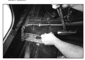
4. Remove the sound deadening on the rear inner wheel well where the rear brace mounting pads will rest.
