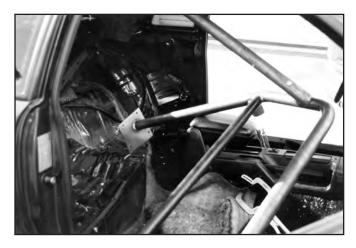
10. Move the driver-side mounting pads into the left rear seat area as you swing the passenger side of the hoop into the car.
