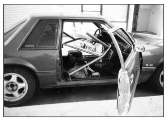
11. Tilt the main hoop upward and rearward to clear the steering wheel.
