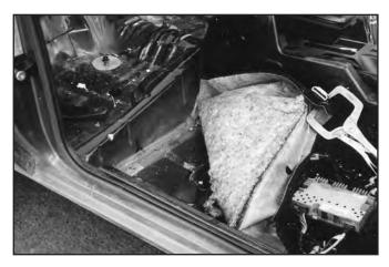
3. Remove excess body seam sealer in the corner where the main hoop mounting pads will rest on the floor pan.
