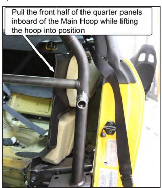
72. Reinstall all the mounting hardware for the main hoop and rear supports before tightening any of the bolts. The main hoop uses 3/8"-16 x 1"-long bolts with a 3/8" G8 washer under the bolt head. The rear supports use 3/8"-16 x 3/4"-long bolts and 3/8" G8 washers beneath the bolt heads.
