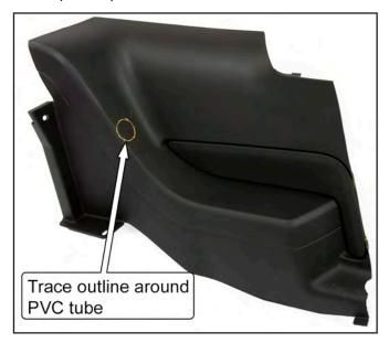
53. Remove the rear half of the plastic panel from the vehicle and hole saw through the location marked for the rear support. Use a 2" hole saw if available, if not a 1-3/4" hole saw can be used and the opening can be filed out larger.
