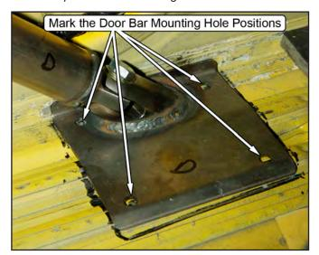
36. Remove the roll bar from the vehicle and drill the four holes marked on each wheel well out to a 7/16" diameter. Use ~1/8" diameter pilot drill to start the holes.
