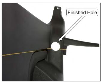
46. Cut the plastic quarter panel into two pieces, along the line that was drawn, using a wood saw or other cutting device.
