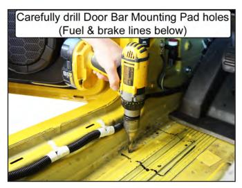
**NOTE:** There ARE fuel and brake lines directly beneath the driver-side door bar mounting pad. Place the door bar doubler plate between the underside of the floor pan and the lines (as a shield) when drilling to prevent puncturing the lines.
