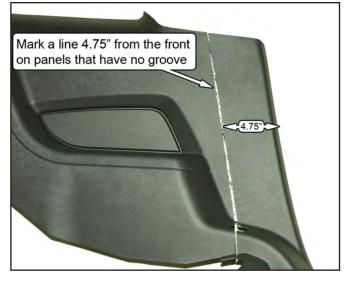
44. At the bottom of the quarter panel, extend the line across the horizontal flat. Add a mark about 3/8" forward of the line, centered side-to-side on the flat section.
