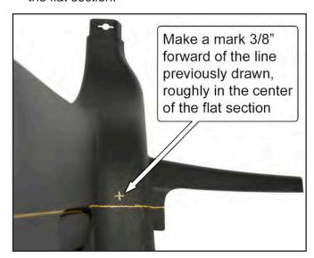
45. Using a 1-3/4" hole saw, cut a hole in the center of the flat, 3/8" forward of the marked line.
