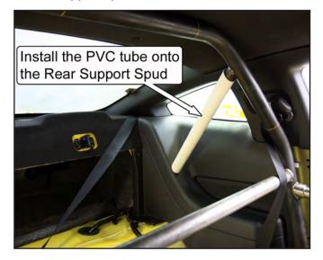
51. Set the roll bar back in its mounting position and slide the PVC tube down until it contacts the plastic quarter panel. Rotate the PVC tube so the end is parallel to the face of the panel.
