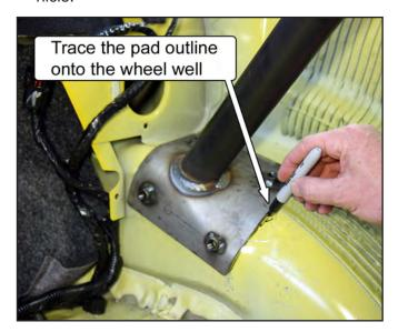
28. Remove the sound-deadening material within the outline using a chisel or other scraping device.
