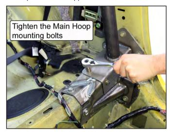
33. With both rear support mounting pads in their proper position (resting firmly against each rear wheel well), tighten the two bolts holding the rear supports to the main hoop so that the rear supports CANNOT move.
