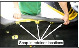
11. Remove the rear quarter panels. There are three (3) push-pin retainers on each panel; one is located at the front of the seat bulkhead and two are at the rear seat backrest. Carefully pull the rear half of the panels inwards to disengage the snap-in retainers located below the quarter window, and then pull the panels forward.
