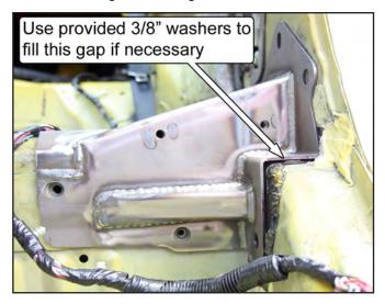
17. Check the gap between the bracket and the vehicle at H8. Use the provided 3/8" G8 washers to close the gap to 1/8" or less. When satisfied, insert one of the factory mounting bolts into the hole to prevent the washers from being dislodged.
