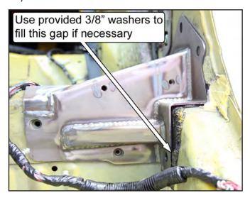
18. Install the remaining mounting bolts into the Support Bracket and tighten them by hand. Take note that H6 and H7 use the larger, 15mm hex head bolts.
