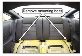
8. Pull the release strap to pivot the backrests down and slide the backrests off of the center pivot bracket to remove them from the car.
