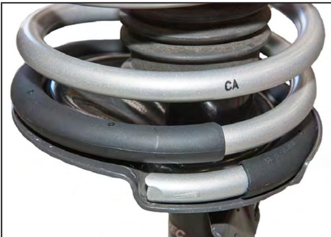
19. Reinstall upper strut mounts or caster/camber plates, ensuring that upper spring completely seats in perch. Torque the strut shaft retaining nut to the OEM torque specification:
