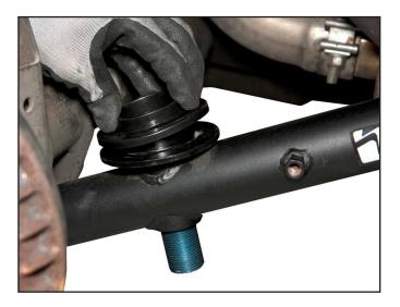
9. Install upper spring isolator on spring.
