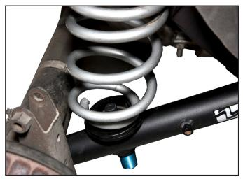
11. Raise the control arm back into place using the floor jack until you can reinsert the rear pivot bolt.
