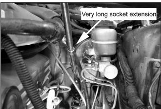
3. Remove the pinch bolt securing the stock steering shaft to the the steering rack input shaft.
