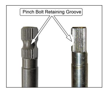
14. Install the lower portion of the MM Steering Shaft assembly onto the input shaft of the steering rack. Orient the lower u-joint so that when inserted, the pinch bolt passes through the retaining groove.
