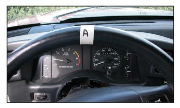
19. Rotate the steering wheel counter-clockwise until full lock is reached. For future reference (in Step 20), count the number of turns required to turn the steering wheel from full lock to full lock.
