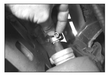
NOTE: Make sure the Lower U-joint pinch bolt is inserted through the unthreaded side of the U-joint first and then into the threaded side. This will allow the U-joint to clamp onto the threaded shaft when the bolt is tightened.
