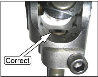
15. Install the pinch bolt removed in Step 9 into the lower U-joint and torque to 24 ft-lbs. The pinch bolt can only be inserted when the lower U-joint is properly positioned on the rack input shaft
