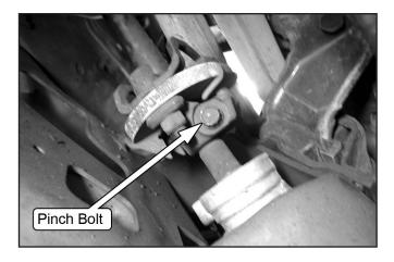
4. Rotate the steering wheel so that the wheels are pointed straight and engage the steering lock so that the steering wheel can't turn.
