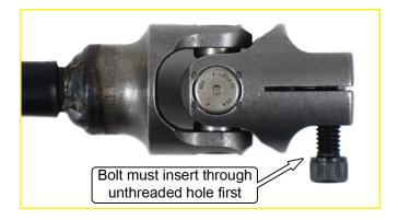
16. Extend the MM Steering Shaft's telescoping section enough to allow the upper U-joint to slip over the splines of the upper stub shaft.
