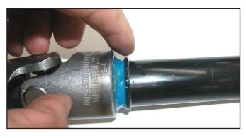
12. Allow the steering shaft to sit for an hour to ensure that the silicone is dry before continuing with the rest of the installation.
