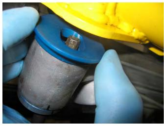
Fully insert the bolt into the k-member rack mounting holes. Make sure the bolt is passing through the correct offset-holes in the rack bushings.
