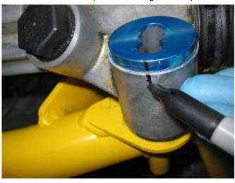
Place the female half of the rear Spherical Rack Bushings into the rear of the rack mounting holes. The concave portion of the bushings should face rearward in the vehicle. Orient the three holes so that they match the orientation of the holes in the front aluminum rack bushings.
