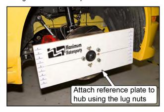
24. Position the reference plate so it is parallel to the ground by using a bubble level or by measuring up from the floor to each end of the plate.
