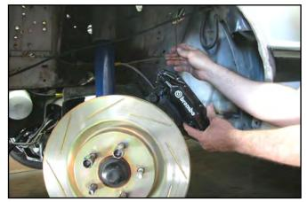
6. Remove the front brake rotor.
