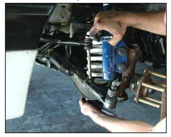
6. Loosen the tie-rod end nut but do not remove it.
