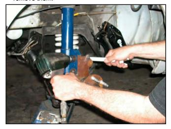
Remove the lower nylock nut from the Tapered Stud and remove the MM Adjustable Tie-Rod End from the steering arm.
