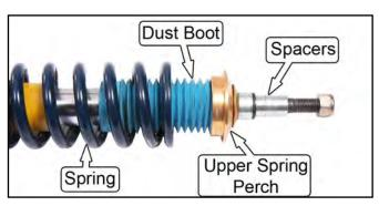
19. Reassemble the spacers and upper spring perch without the spring, dust boot, or external bumpstop, and reinstall the strut back onto the car in the reverse order of removal.
