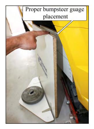
28. The dial indicator and the fixed pointer must be attached to the bumpsteer gauge at this point. When viewing the gauge from the side of the vehicle, attach the dial indicator to the rearward edge of the bumpsteer gauge and attach the fixed pointer to the forward edge of the bumpsteer gauge by hand tightening the clamp bolts. The pointers should be facing the reference plate.
