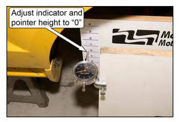
30. When looking down at the top of the bumpsteer gauge and the top of the reference plate, the two edges should be parallel to each other. This will center the dial indicator in its travel range. Pivot the base of the bumpsteer gauge either towards or away from the reference plate to make them parallel within 1/4" of each other.
