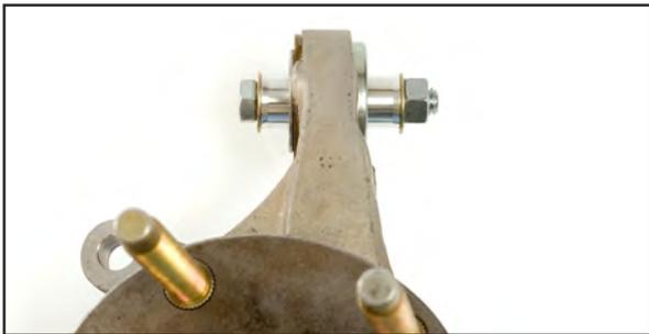
25. Draw the Bearing Insert into the spherical bearing by tightening the bolt with a pair of wrenches. Make sure the Insert seats flush against the face of the spherical bearing.
