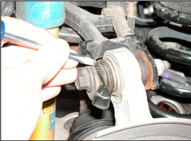
4. Remove the control arm mounting bolt securing the cross-axis joint that needs to be replaced.
