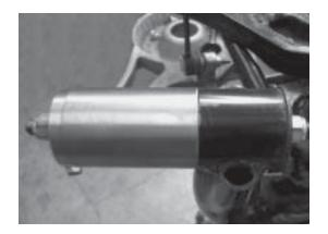
18. With a deep socket placed on the inboard nut, slowly tighten the outboard nut, making sure that the small removal disk is centered within the bushing shell. Continue to tighten the nut until the bushing is pulled free of the bushing shell.
